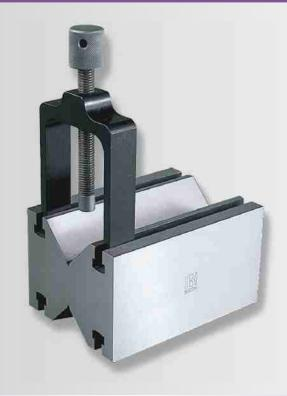
**Prism with clamp** made from hardened, stabilised stainless steel. Entirely ground. With two 90° "V"s. Manufactured to tolerances of planarity and parallelism <=0,005 mm. Supplied singly.
