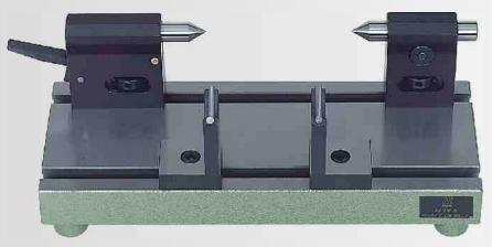
Universal table for shaft control. Cylindrical items can be controlled. Assembled with the appropriated parts, diameters, conicities, lengths and concentricities can be controlled. Two "V" blocks or two tailstocks following the design of the piece to control, can be slide on precision hardened and ground T-slot.
