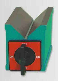
Magnetic V-block. Suitable for anchoring items of different shapes. Indispensable for grinding, milling and scribing jobs. Fitted with locking lever. Manufactured to tolerances of planarity and parallelism ±0,01 mm. With two 90° "V"s. Supplied in case.
