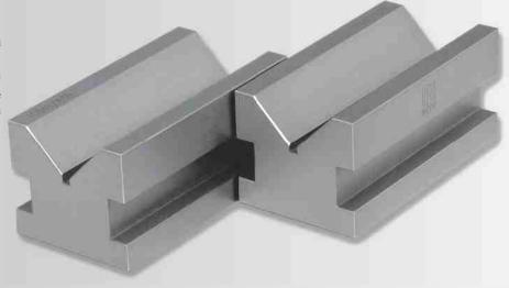
Right angle V-block made from ground G25 perlitic cast iron. Manufactured to tolerances of planarity and parallelism as per DIN 2274. Supplied in pairs.
