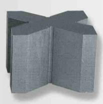
High precision V-blocks. Made from hardened, stabilised stainless steel. Entirely ground. With four 90° "V"s. Manufactured to tolerances of planarity and parallelism <=0,005 mm. Supplied in pairs.
